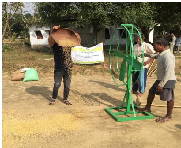
Fig. 4: Demonstration of hand operated winnower
